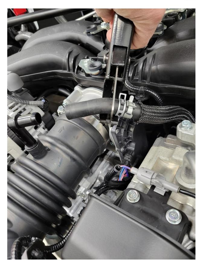
Step 5. Install Killer B Motorsport AOS with downward inlet port. The hoses may fit tightly. If you need to, use a drop of dish detergent or oil to help with install.
