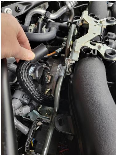
Step 7. Install Killer B Motorsport AOS with flanged ports. The hose on the Manifold port fits
