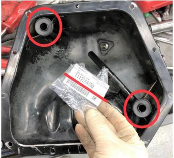
Install two new "sealing o-rings": 11122AA350.
