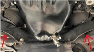
With a 10mm socket, socket wrench, extension and swivel adaptor, loosen ALL ELEVEN of the M6 oil pan mounting bolts:
