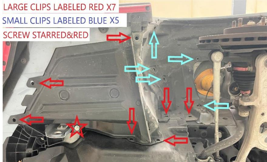
8. Use a bungee cord to pull the liner back toward the wheel hub, exposing the reservoir.
