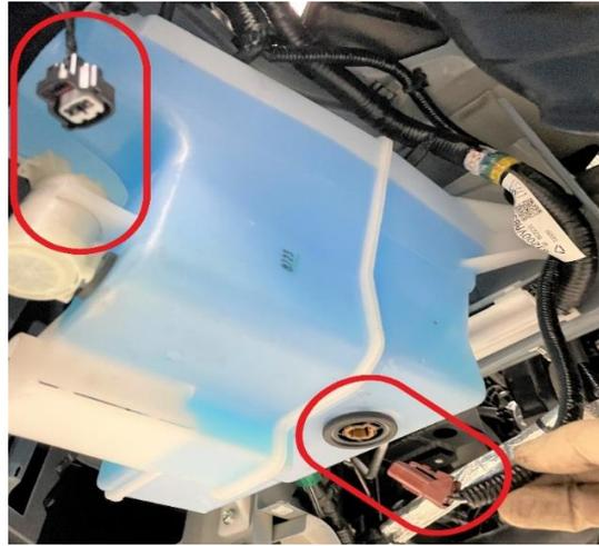
10. Use a bucket to catch any washer fluid if you want to reuse it. (use a coffee filter to filter out contaminants).
