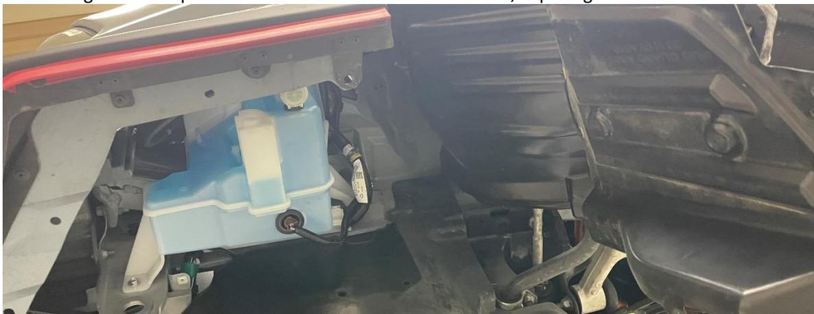
9. Unplug the washer fluid pump and low fluid warning float.
