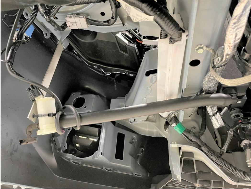
26. Pour a couple of ounces of water in the WASHER side of the Killer B reservoir and check for leaks. Make sure that grommet did not deform when you inserted the elbow.
