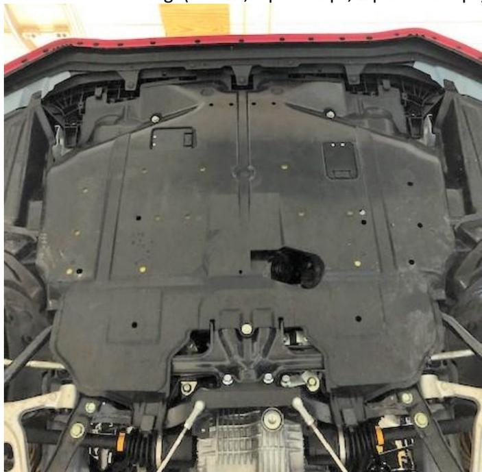
32. Mark your belly pan for trimming, to allow clearance for the 5/8" ID hose.
