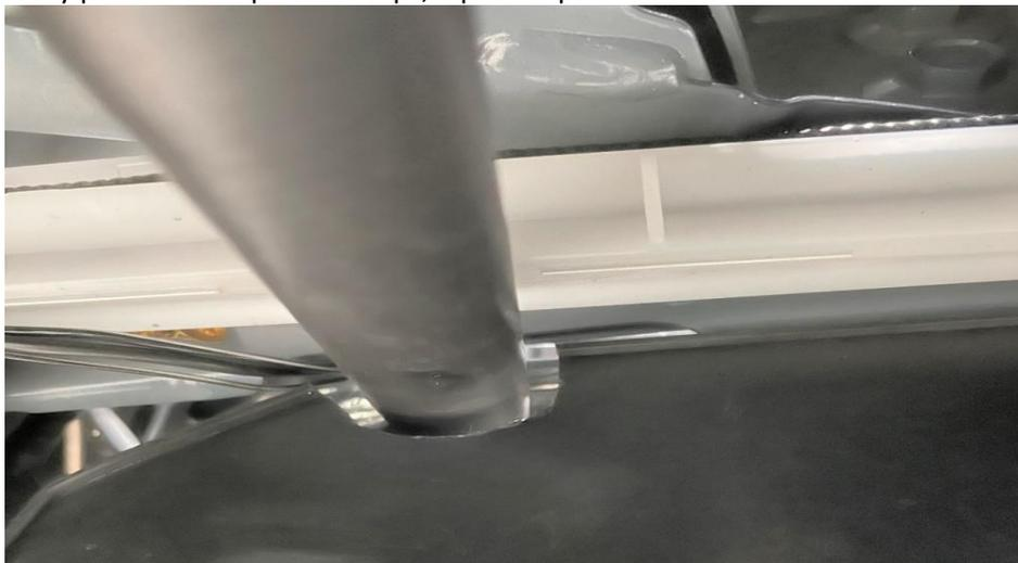
34. Check for obstructions and then lower the vehicle to the ground.
