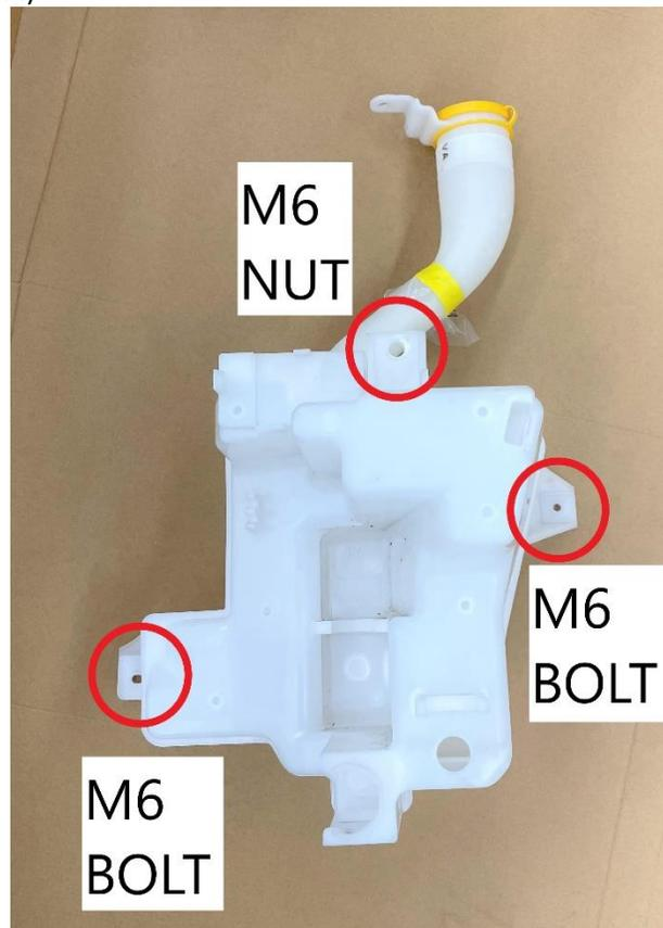
15. Remove the factory washer fluid reservoir.
