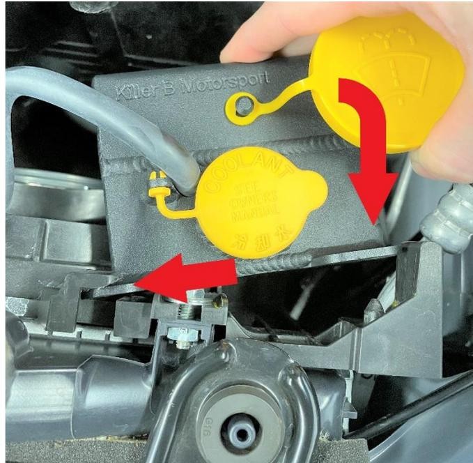
NOTE for 2019+ models: If you can see that the radiator shroud is curved after installing the reservoir, remove the reservoir and trim more from the shroud so that the shroud is not stressed from having the reservoir installed.
