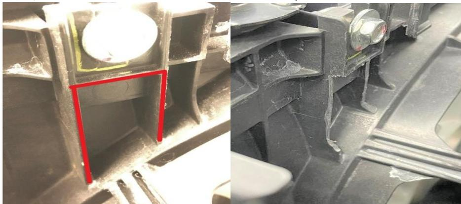
5. Use a screwdriver to loosen the clip from the filler neck of the washer fluid reservoir.
