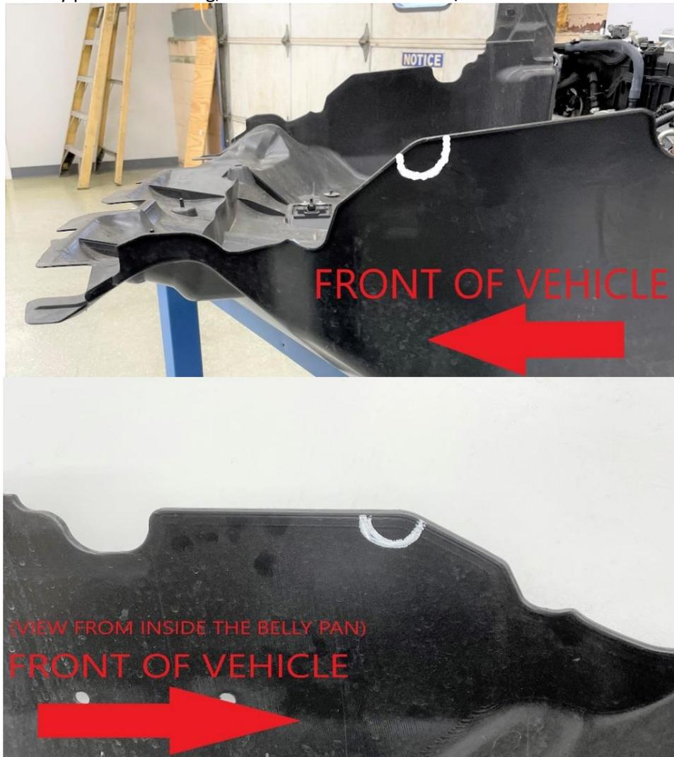
33. Reinstall belly pan: install 2 plastic C clips, 6 push clips and 3 bolts.
