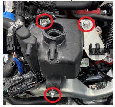
4. Identify and remove the two 1/2" coolant hoses for the reservoir.
