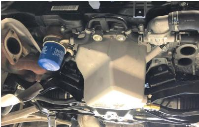
27. Lower the jack that is pushing the trans/engine up. This should lower the engine mount studs back through the holes in the engine cradle. Make sure the engine is centered (left to right) in the cradle before installing and torqueing the mounting nuts. Passenger's sideDriver's side-
