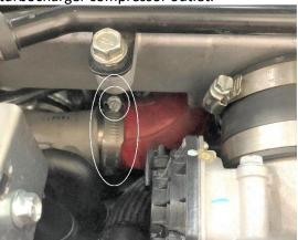
8. Next, loosen the upper worm clamp (closest to the intercooler).
