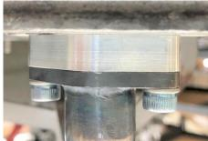
21. Grab the second and third oil pickup spacers from the parts kit and install them between the engine block and the oil pickup bracket. Install the (2) black bolts through the pickup and through the spacers. Now that all pickup and baffle hardware is loosely threaded into place, turn them clockwise by hand until they all become seated. Using a torque wrench, tighten the oil pickup and baffle hardware to 7.5 ft-lbs (90 in-lbs).
