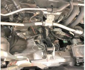
11. Pull the dipstick up 2 inches or remove it completely. Loosen the oil fill cap and raise the vehicle to drain the oil.
