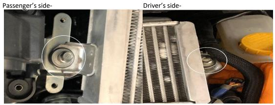
4. With the same tools, remove the two bolts securing the PCV balance pipe to the intercooler.
