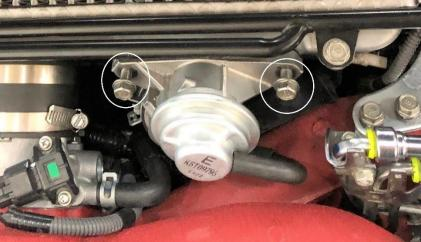
6. With the same 12mm socket and socket wrench, remove the two remaining bolts securing the driver's side intercooler bracket to the intake manifold.
