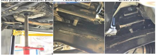
15. You may now begin unfastening the (14) mounting bolts securing the engine oil pan to the engine block. You will need a 10mm socket and socket wrench and a swivel to access all OEM pan hardware.
