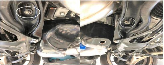
14. We recommend removing the pre-turbo exhaust heat shields, the driver's side exhaust manifold section and the center crossover pipe. This will provide you with the necessary amount of space required for pan removal. Be sure to replace the exhaust gaskets that you remove, they are single use only.
