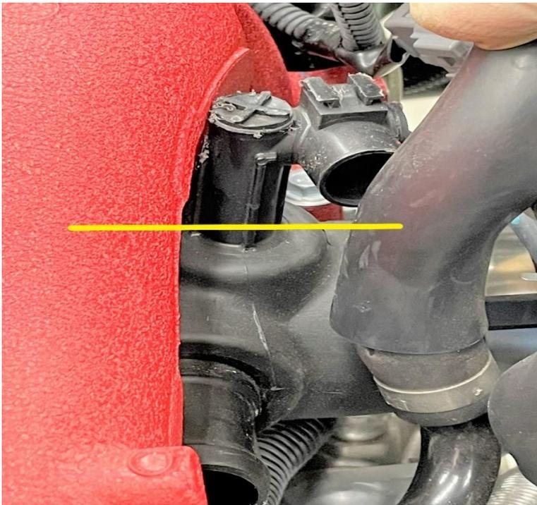
12. Remove the down-ward facing M6 bolt with a 10mm tool. This will help you push the Killer B inlet past the factory hard fuel lines. Reinstall once you have
