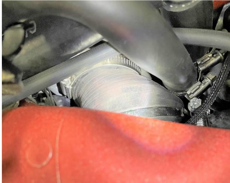
13. Tighten the clamp that secures the turbocharger inlet coupler to the turbocharger.
