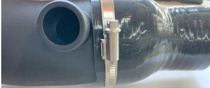
2. Install the turbo inlet on the engine and note where the mounting tab on the turbo inlet sits in relation to the intake manifold. Make sure you clock the coupler appropriately as well.
