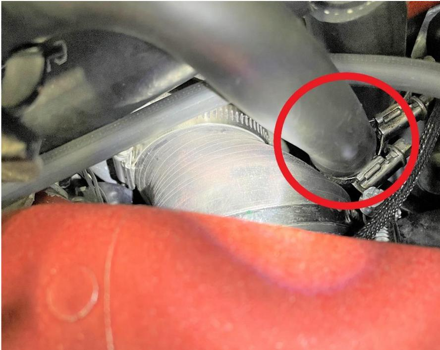
3. Remove/cut a small amount at a time starting with 1/8" cuts. Repeat the procedure until you have a finished result with no kinks, pinches or bends in the coupler.
