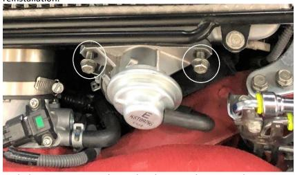
6. With the same 12mm socket and socket wrench, remove the two remaining bolts securing the driver's side intercooler bracket to the intake manifold.
