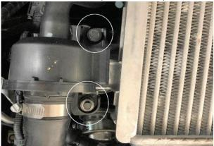
3. With a 12mm socket and socket wrench, remove the bolts on the driver and passenger side of the intercooler.
