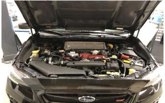
This installation requires temporary removal of your intercooler and pitch mount. This allows you to raise the engine up from the cradle.
