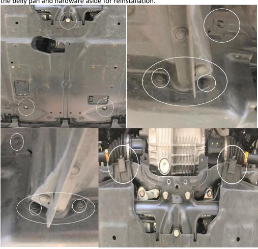
13. Drain the engine oil for as long as possible. The longer it drains, the cleaner your workspace will remain. We recommend changing the filter as well. While the oil drains, remove the two nuts (and washers, if applicable) securing the bottom side of the engine mounts to the engine cradle. Passenger's side:
