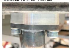
21. Grab the second and third oil pickup spacers from the parts kit and install them between the engine block and the oil pickup bracket. Install the (2) black bolts through the pickup and through the spacers. Now that all pickup and baffle hardware is loosely threaded into place, turn them clockwise by hand until they all become seated. Using a torque wrench, tighten the oil pickup and baffle hardware to 7.5 ft-lbs (90 in-lbs).
