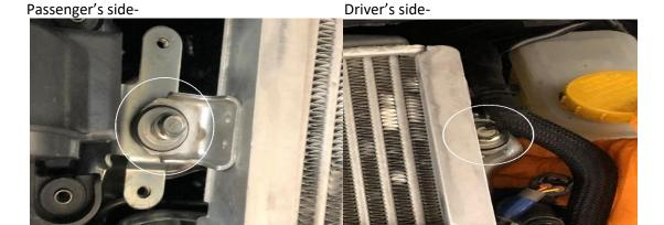
4. With the same tools, remove the two bolts securing the PCV balance pipe to the intercooler.
