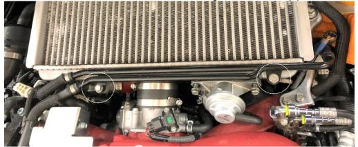
5. Remove the two bolts securing the bypass valve to the intercooler. Set all bolts aside for reinstallation.
