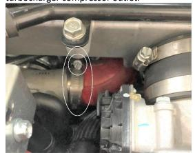
8. Next, loosen the upper worm clamp (closest to the intercooler).
