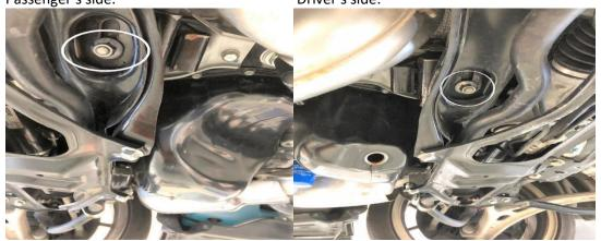
14. We recommend removing the pre-turbo exhaust heat shields, the driver's side exhaust manifold section and the center crossover pipe. This will provide you with the necessary amount of space required for pan removal. Be sure to replace the exhaust gaskets that you remove, they are single use only.
