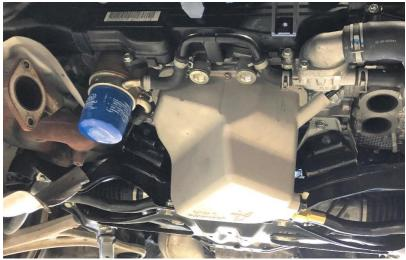
27. Lower the jack that is pushing the trans/engine up. This should lower the engine mount studs back through the holes in the engine cradle. Make sure the engine is centered (left to right) in the cradle before installing and torqueing the mounting nuts.
