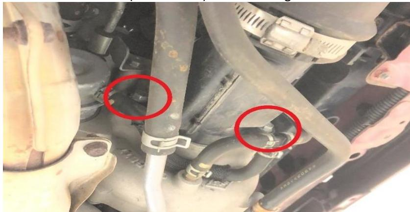
Loosen and remove the 2 M8 bolts securing the charge pipe to the compressor outlet flange:
