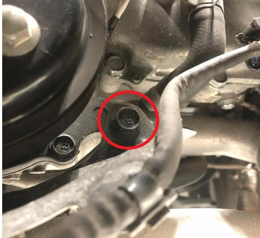
Unfasten the J-pipe from its front (4) nuts and rear (2) nuts/bolts:
