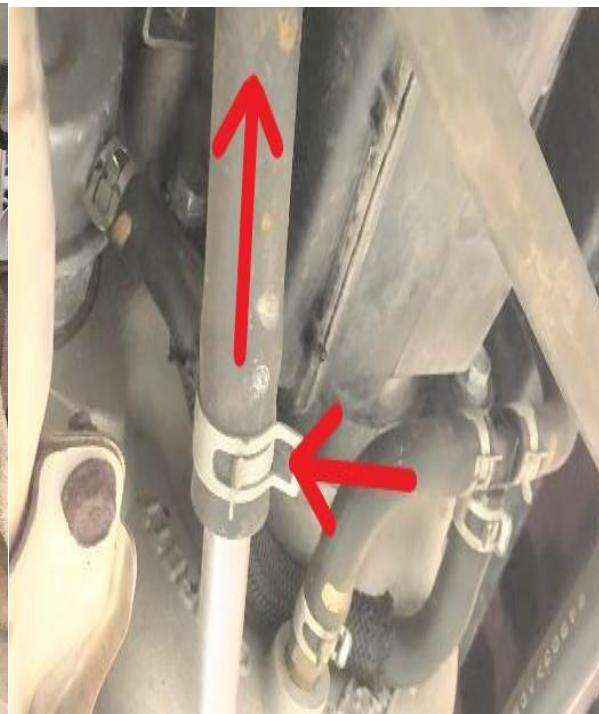
Remove the coolant feed and coolant drain lines from the turbocharger.
