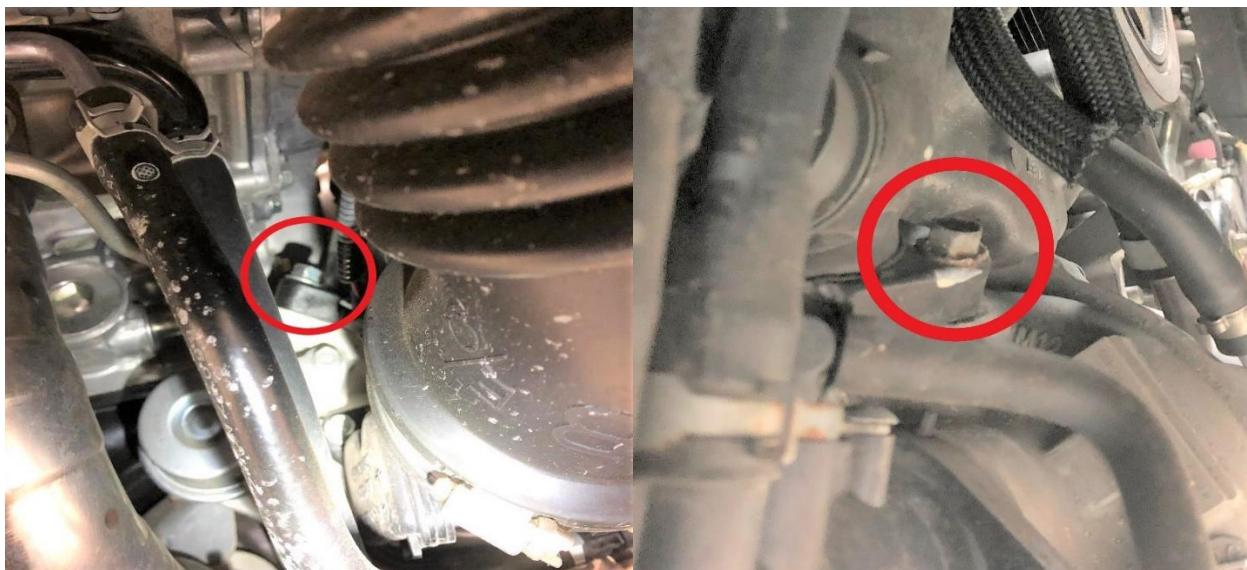
Loosen the air duct that attaches to the turbocharger inlet. Remove and set aside:
