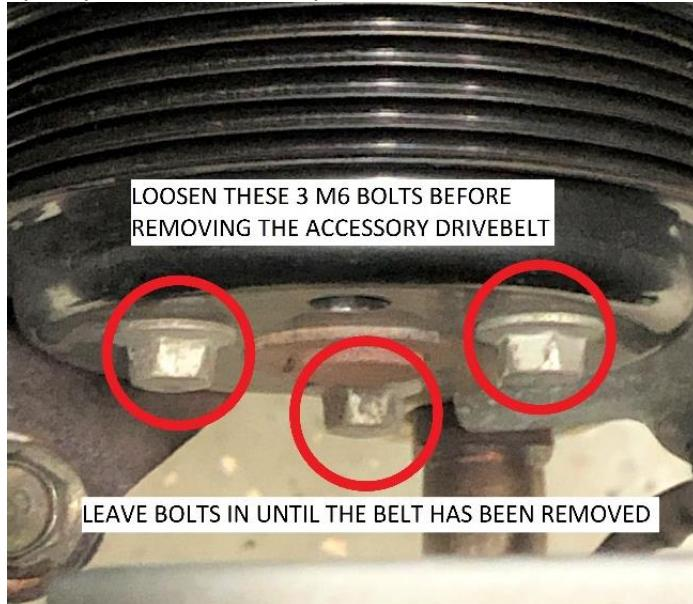
Use a piece of paper and pen to illustrate the accessory belt routing or refer to the factory service manual. Remove the accessory drive belt using a 14mm wrench or socket wrench [Some models may use a 15mm]: Install wrench or socket wrench near the 1:00 or 2:00 position and then rotate clockwise to take the tension off the belt.
