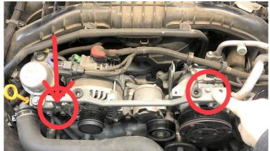
7. Loosen the (4) M12 bolts securing the AC compressor to the engine block. Set 4 bolts and bracket aside for reinstallation. Once you are able to lift the AC compressor vertically, spray compressed air under the compressor to remove dust and debris from your work area.
