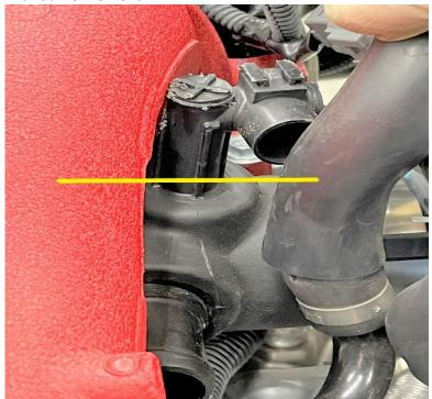
12. Remove the down-ward facing M6 bolt with a 10mm tool. This will help you push the Killer B inlet past the factory hard fuel lines. Reinstall once you have
