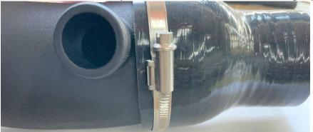
2. Install the turbo inlet on the engine and notate where the mounting tab on the turbo inlet sits in relation to the intake manifold. Make sure you clock the coupler appropriately as well.
