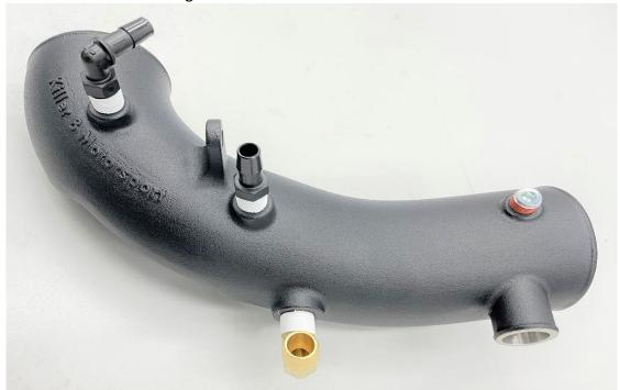
CAUTION: When threading each NPT (tapered) fitting, watch carefully inside the inlet. Thread each fitting in until the threads of each fitting just start to stick through the inside of the inlet. While doing so, be sure to position the elbow fittings to their correct location.
