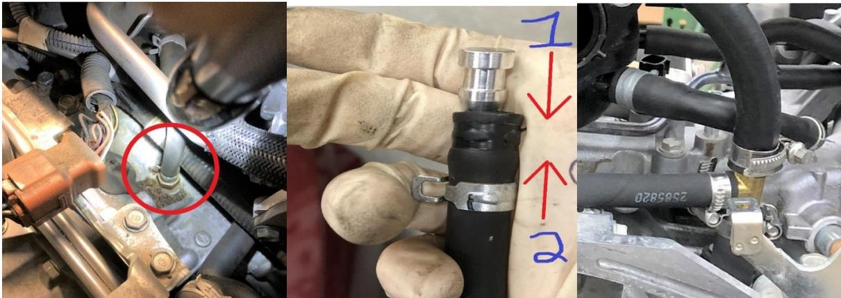
13. Using a 19mm deep well socket, swivel adaptor, extension, socket wrench- loosen and remove the PCV valve.
