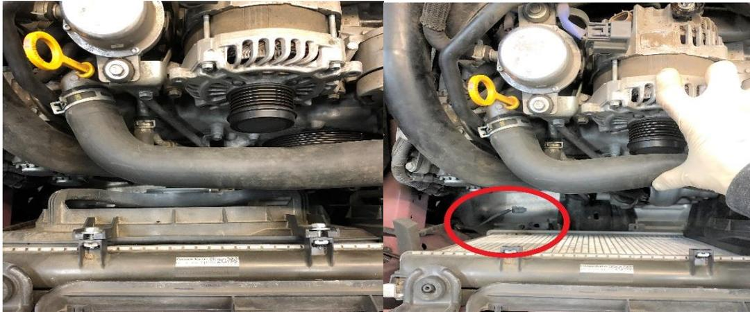
10. Locate the (4) 14mm headed bolts that secure the AC compressor to the engine block. Two will be vertical and the remaining two will be facing the front of the vehicle. Loosen and remove these (4) bolts and set aside. Also, set bracket aside for reinstallation. **DO NOT LOOSEN/DISCONNECT ANY REFRIGERANT LINES.** Pick up the compressor and set it on top of the tensioner so you can access the factory coolant/ breather assembly.
