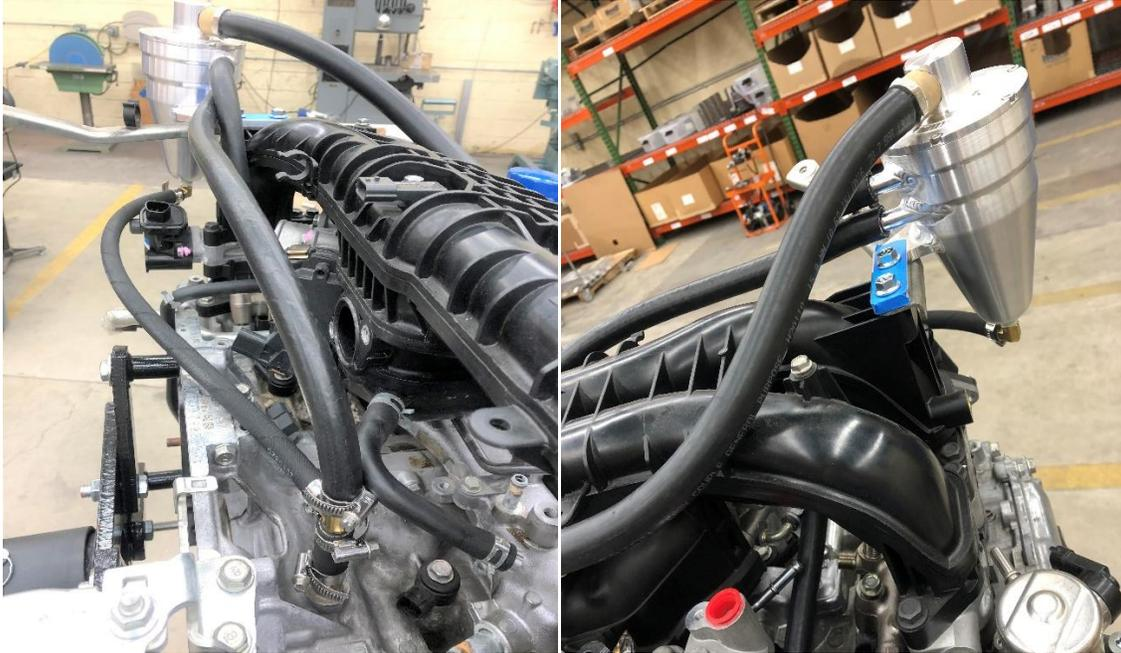
27. Install the free end of the 3/8" drain hose on the drain elbow of the AOS with the last small hose clamp. Tighten the clamp.
