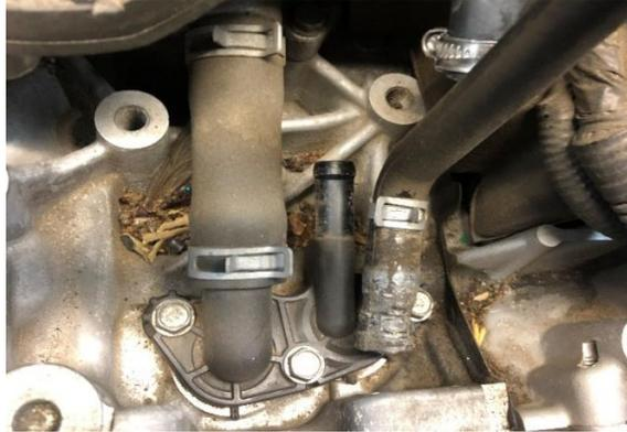
12. Locate the PCV valve and hose on the top of the engine. It is behind the intake manifold, on the passenger's side. Use pliers to loosen the hose clamp, slide it up the hose about an inch, lift the hose from the PCV valve. Remove the clamp. Grab the supplied hose plug and install it in the vacuum hose. Install the supplied SMALL zip tie to secure the plug in place. Tuck the plugged hose away so that it does not interfere with the remainder of this install.
