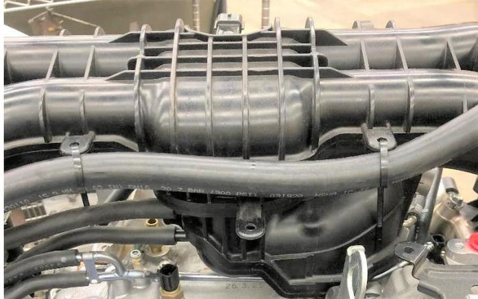
You may need to cut a small slot in the driver's side of your engine cover to allow clearance for the AOS suction hose.
