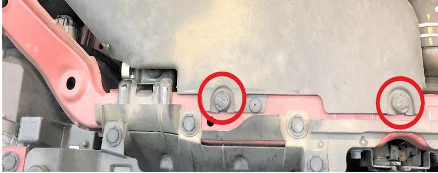
9. Unplug the passenger's side radiator fan and then loosen/remove the (2) 10mm headed bolts securing the fan to the radiator. Remove the fan from the vehicle. Set aside.
