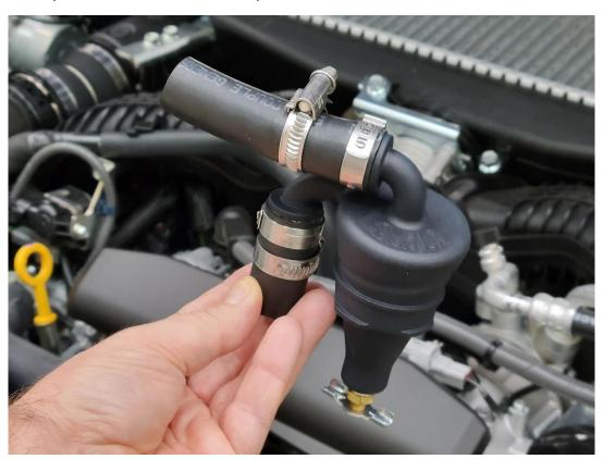
Step 5. Install AOS Hoses as shown onto the factory tubes. Tighten Worn Drive Hose Clamps.
