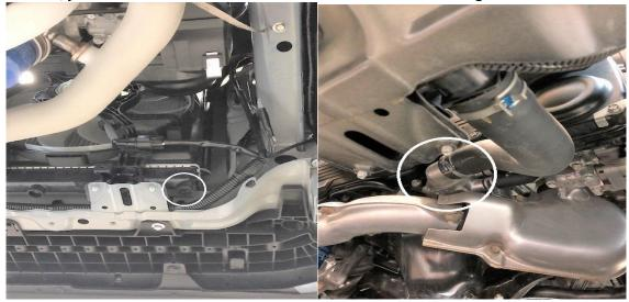
4. Once the coolant has been drained; using pliers, decompress the two clamps securing the hose to the radiator and water pump inlet. While the clamps are compressed, slide them toward the center of the hose for now. You may need a run a small pointed pick around the edges of the hose to work it free.
