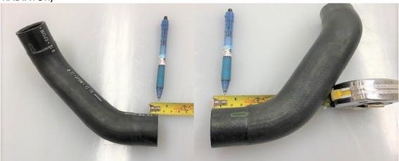
The following photograph shows the correct orientation of the lower radiator hose. The yellow arrow should now be opposing coolant flow. This will not affect the functionality of the cooling system.
